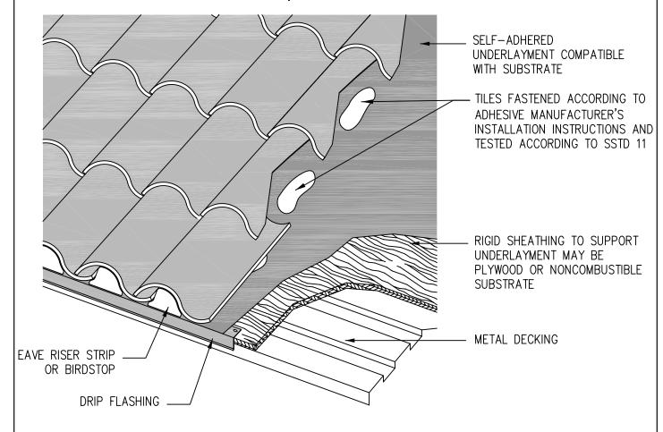
Note: Attachment of underlayment to sheathing shall be in accordance to assemblies that have been tested to SSTD 11.
