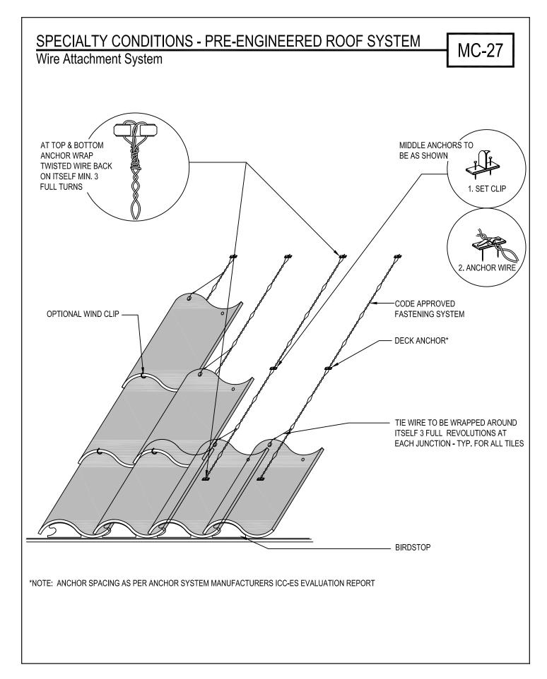
DRAWING SHOWN DEPICTS THE APPLICATION OF ALL TILE PROFILES. UNLESS OTHERWISE NOTED IT WOULD APPLY TO EITHER CONCRETE OR CLAY TILES.
