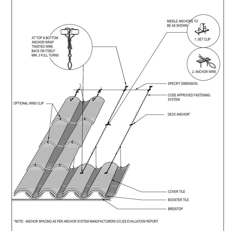
DRAWING SHOWN DEPICTS THE APPLICATION OF ALL TILE PROFILES. UNLESS OTHERWISE NOTED IT WOULD APPLY TO EITHER CONCRETE OR CLAY TILES.
