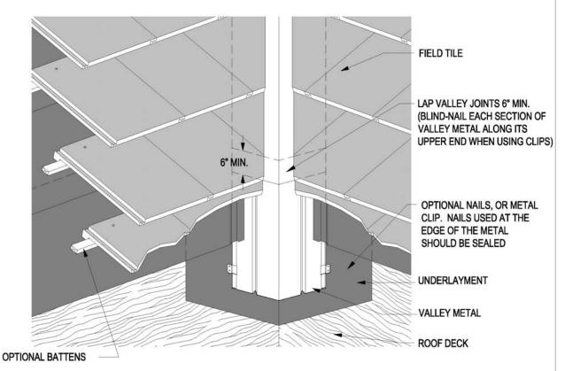
Note: Tile at valleys may be cut to form closed or open metal valley detail. When flat profiled tile is installed as "closed valley" a ribbed valley metal or a single crown valley metal with a batten extension shall be used.
