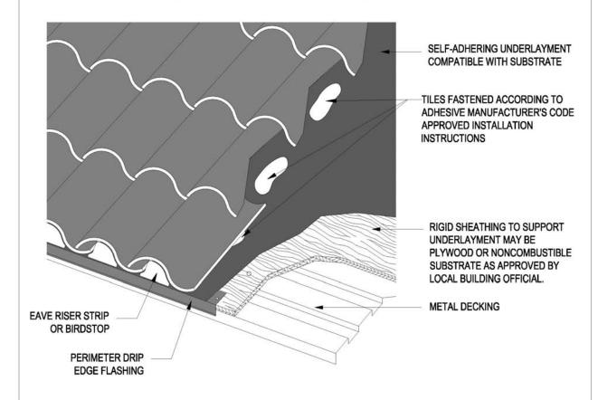
Note: Adhesion of underlayment to substrate shall be in accordance with assemblies recognized in a current ICC-ES evaluation report for roof tile adhesives evaluated to the requirements of AC-152.
