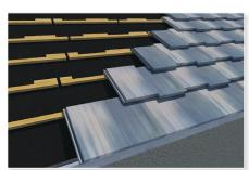
If battens are to be used, the stagger is achieved by installing partial battens immediately above the standard battens from the second Course up. The tiles with the shorter exposure will hang on the higher partial batten (see image). If no battens are used, a second set of lines will be marked at each Course, one line for the normal exposure and one for the staggered tiles.
