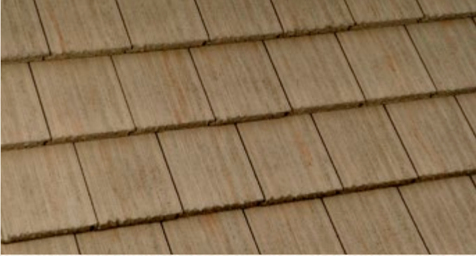
5530 Weathered Adobe - Hues of Tan, Rust Streaks Ref: .23 Emi: .92 SRI: 24 A.SRI: 27 CRRC: 0918-0017
