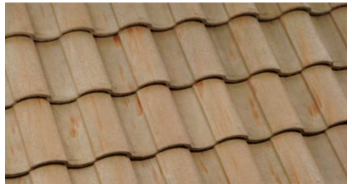
3530 Weathered Adobe - Hues of Tan, Rust Streaks Ref: .23 Emi: .92 SRI: 24 A.SRI: 27 CRRC: 0918-0017
