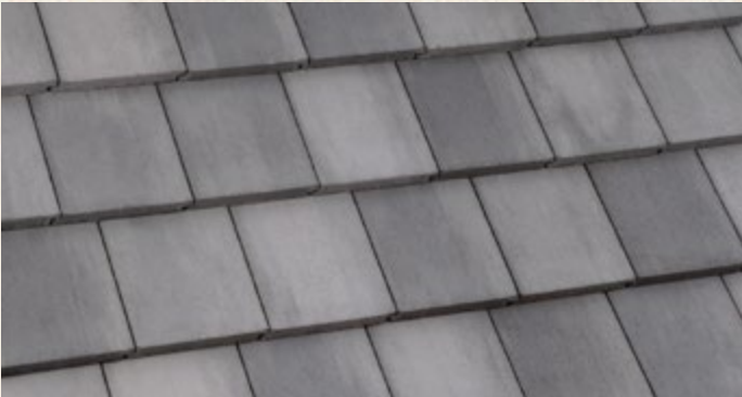
4679 Light Gray Range - Range of Light Gray Ref: .21 Emi: .93 SRI: 22 A.SRI: 21 CRRC: 0918-0004
