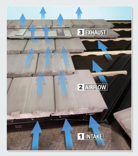
**The Ventilated Roof System** is an all-in-one concrete tile roof system that focuses on energy efficiency, savings and performance. It is comprised of three key elements that revolve around facilitating airflow.
