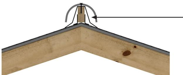
Mechanically Attached Wood Hip and Ridge Boards Using Metal Brackets. Cover with Self-Adhered Weather Blocking.
