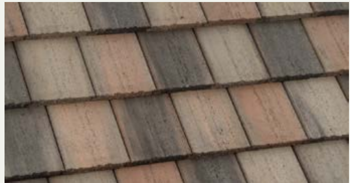
SHE 8773 Walnut Creek Blend - Blend of Tan, Orange, Dark Brown CRRC 0918-0037 Ref .20 EMI .94 SRI 21 A.Ref .23 A.EMI .91 A.Sri 23
