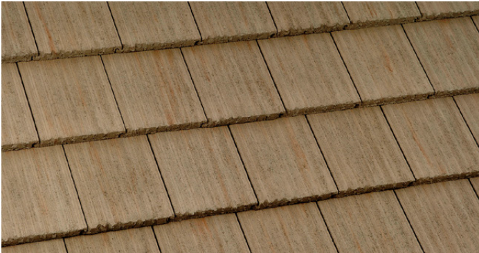
330 Weathered Adobe - Range of Tan, Rust Streaks CRRC 0918-0017 Ref.23 Emi.92 Sri 24 A.Ref.26 A.Emi.90 A.Sri 27
