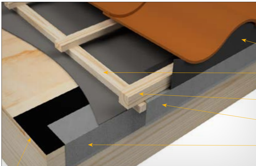
HIGH PROFILE TILE WITH BIRD STOP
